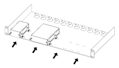
Step 4 Install the rack in a cabinet.
