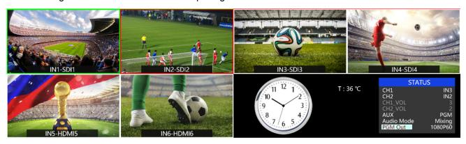
The lower right two sections display time, menu and status information. The CH1,CH2 are the channel selection of the 2 audio sources for audio mixer.
