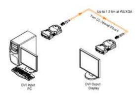
Figure 1 - Schematic Connection Diagram of Optical DVI Extension Modules
