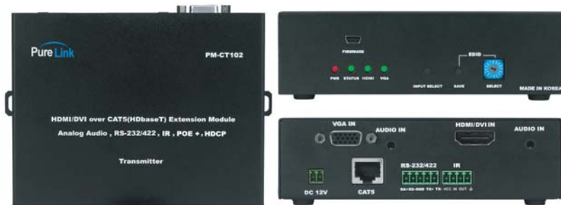
PM-CT102: PM series HDMI over CAT5e (HDBaseT) Extender Transmitter
