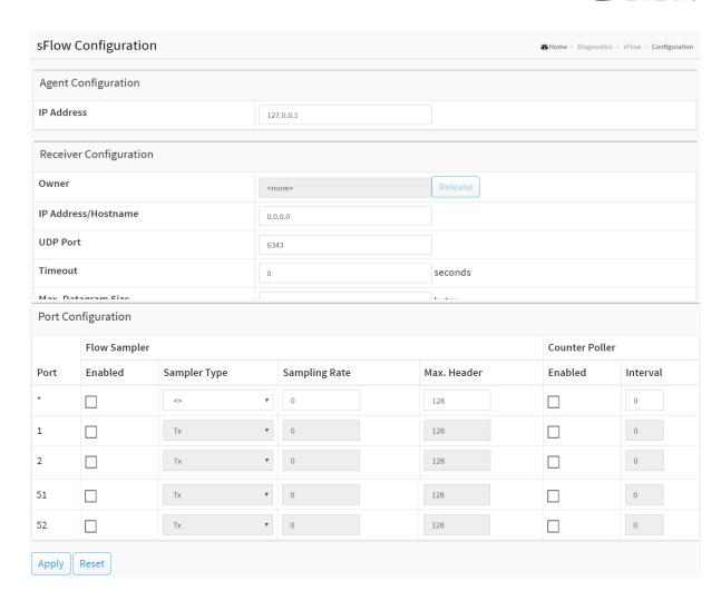
Figure 15-5.1: The sFlow Configuration
