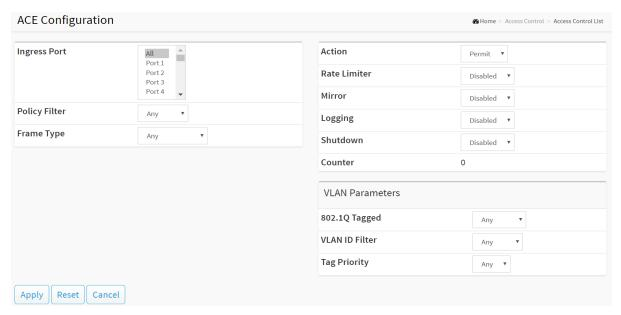
Figure 12-3: The Access Control List Configuration
