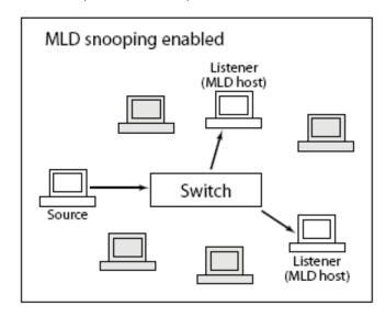
Figure 9-2: The MLD snooping enable
