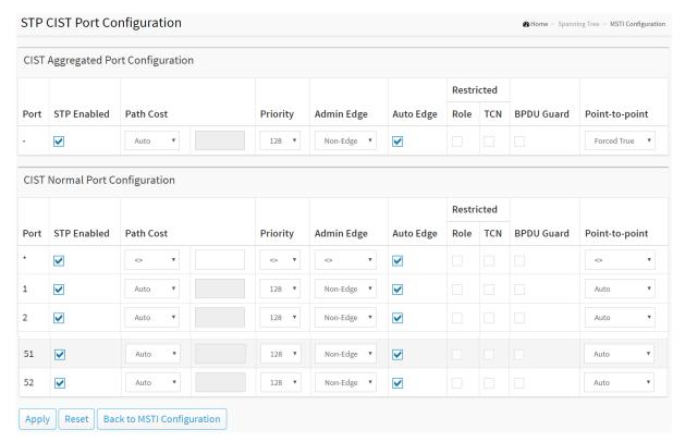
Figure 7-2: The STP CIST Port Configuration
