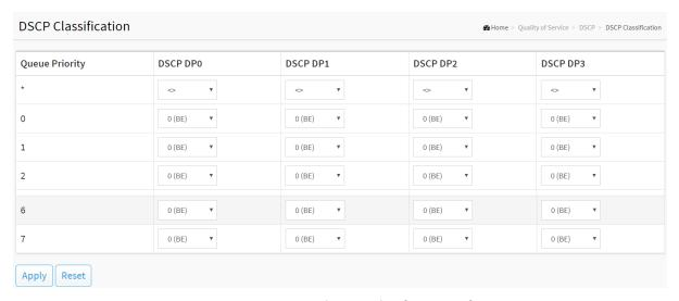
Figure 6-7.3: The DSCP Classification Configuration
