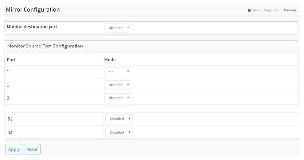
Figure 15-4: The Mirror Configuration
