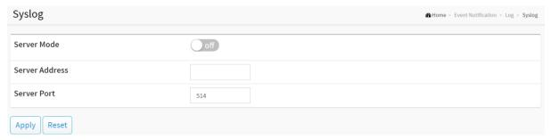
Figure 14-3.1: The System Log configuration
