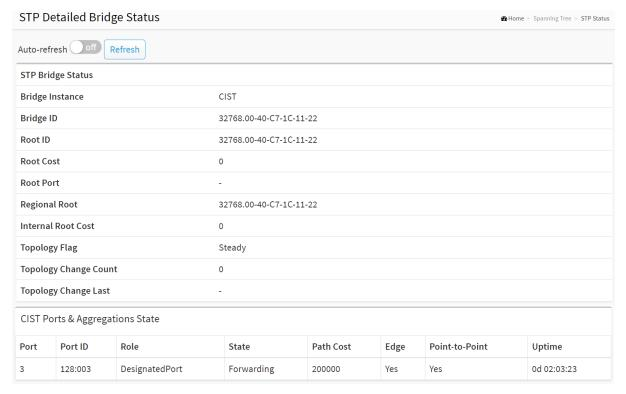
Figure 7-3: STP Detailed Bridge Status
