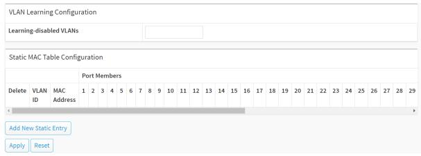
Figure 8-1: The MAC Address Table Configuration
