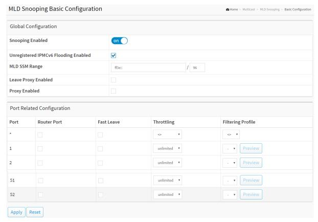
Figure 9-2.1: The MLD Snooping Basic Configuration
