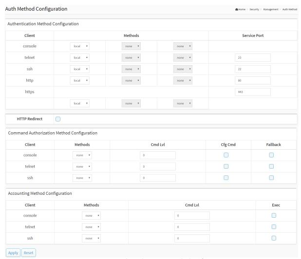
Figure 11-1.3: The Authentication Method Configuration
