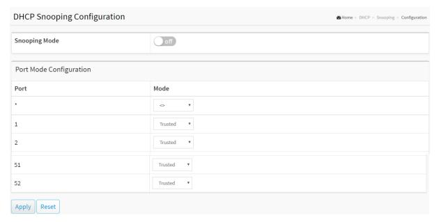
Figure 10-1.1: The DHCP Snooping Configuration
