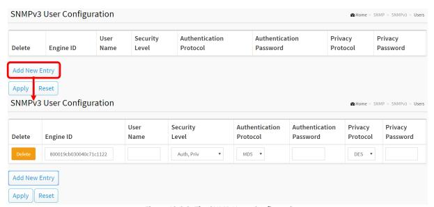
Figure 13-2.2: The SNMP Users Configuration
