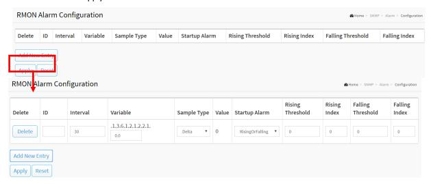
Figure 13-5.1: The RMON Alarm Configuration
