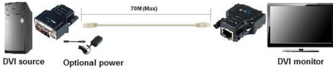
Figure 1 – Schematic Connection Diagram of DCE II Tx/Rx
